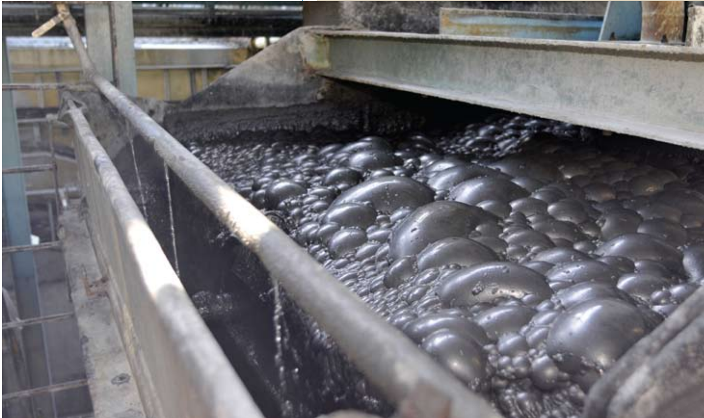
Concentrate flotation froth
